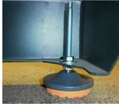
Figure 5: Machine base (foot) - mounting on the baseplate
