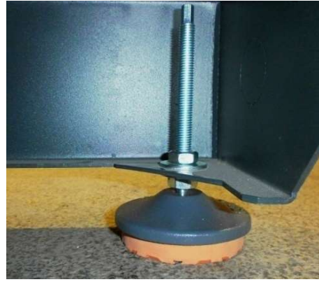
Figure 5: Machine base (foot) - mounting on the baseplate
