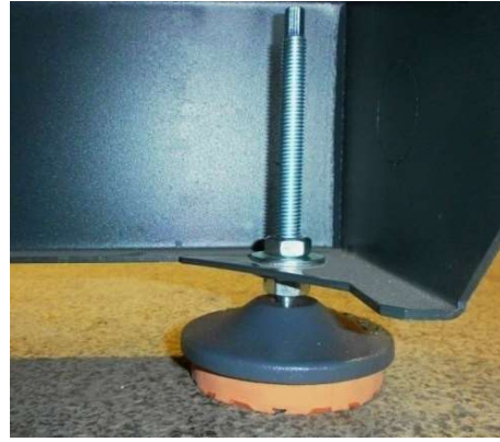
Figure 5: Machine base (foot) - mounting on the baseplate
