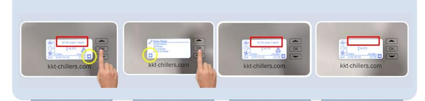
If a fault is present, it can be read above the temperature read out.
