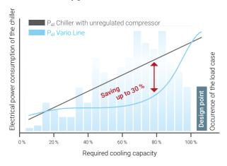
As a result, not only the reduced noise emission is noticeable. Due to the lower power consumption when operating under partial load, use of the Vario-Line can lower operating costs significantly.
