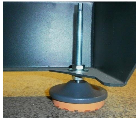
Figure 7: Machine base (foot) - mounting on the baseplate
