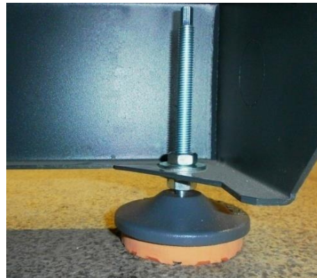
Figure 6: Machine base (foot) - mounting on the baseplate
