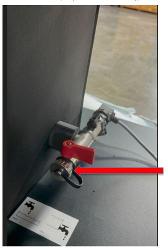
bottom connection port with the redhandled ball valve. **Note: 3/8" BSPP male threaded connection**
